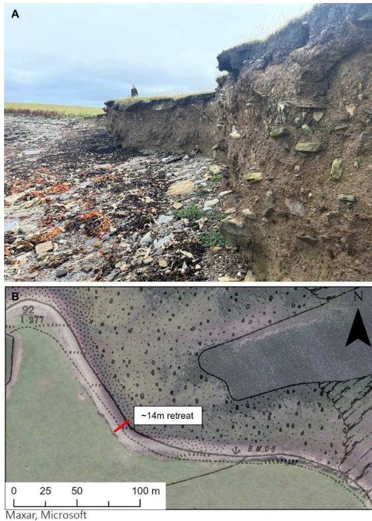
Figure 7A. Erosion of coast edge on northern side of Grice Ness. Figure 7B. Comparison of coast edge using modern satellite imagery and 1900 historic mapping (1:2500 County Series 1 st Revision [TIFF geospatial data], Scale 1:2500. Tiles: orkn-hy6728-2.tif, Updated: 30 November 2010, Historic, Using: EDINA Historic Digimap Service, https://digimap.edina.ac.uk , Downloaded 2023-10-09).
