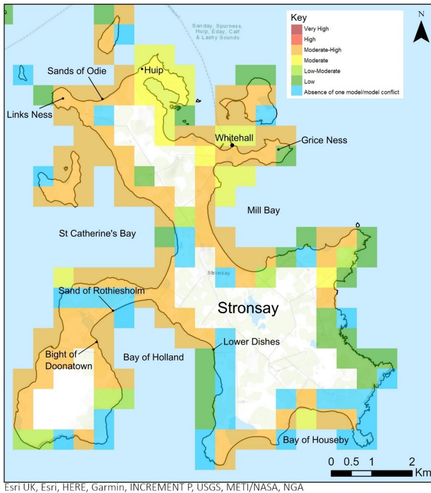
Figure 2. Modelled vulnerability of the Stronsay coastline. Red, orange and yellow cells denote coast which is experiencing erosion and therefore targeted during the 2023 CCZAS survey. Green cells denote coast that is not experiencing erosion and blue cells denote areas where there is a conflict between the models, or which are only included by one model.
