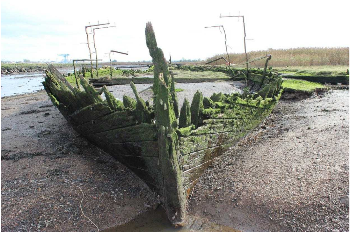
Figure 25: General view of schooner 9 from stem, facing south. Iron L-shaped knees indicate deck height.
