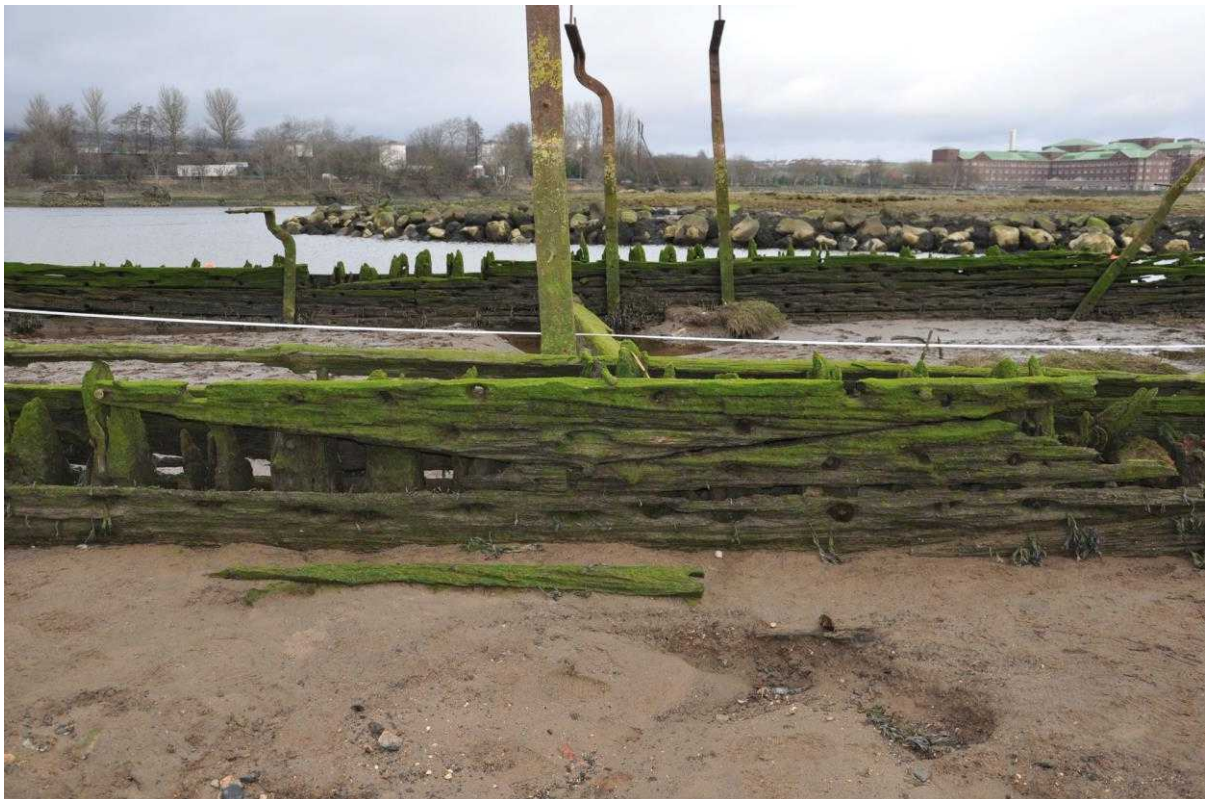
Figure 28: Detail of scarf repair to planking on port side of schooner 9.
