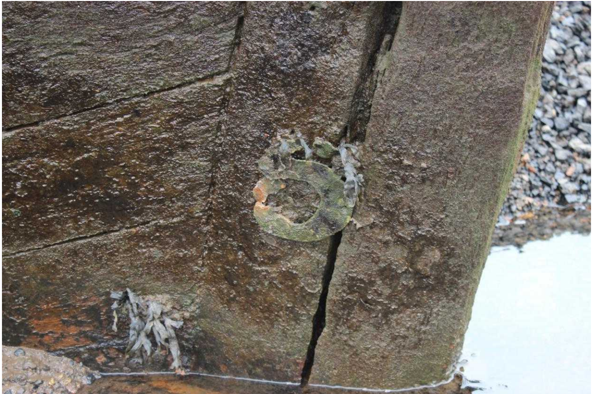
Figure 27: Detail of draft mark on stem post of schooner 9 indicated by lead numeral 5.
