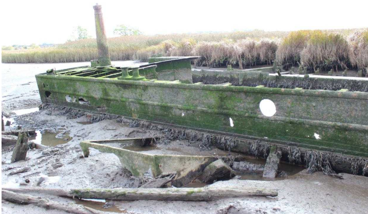
Figure 17: Diving Bell Barge, starboard side, showing upturned remains of diving bell next to hull, and the mooring bollards.
