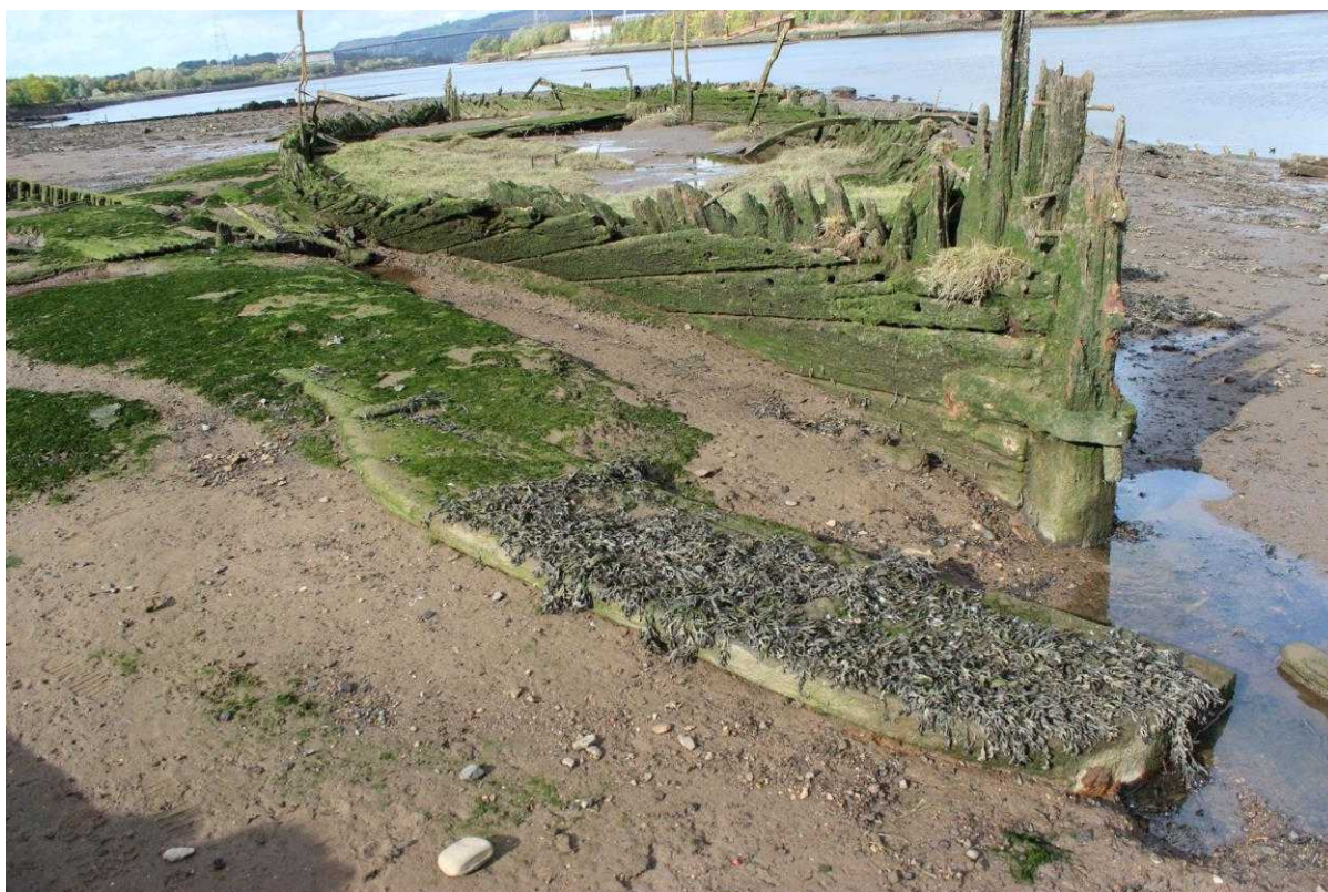
Figure 30: Detail of detached rudder adjacent to stern post of schooner 9.
