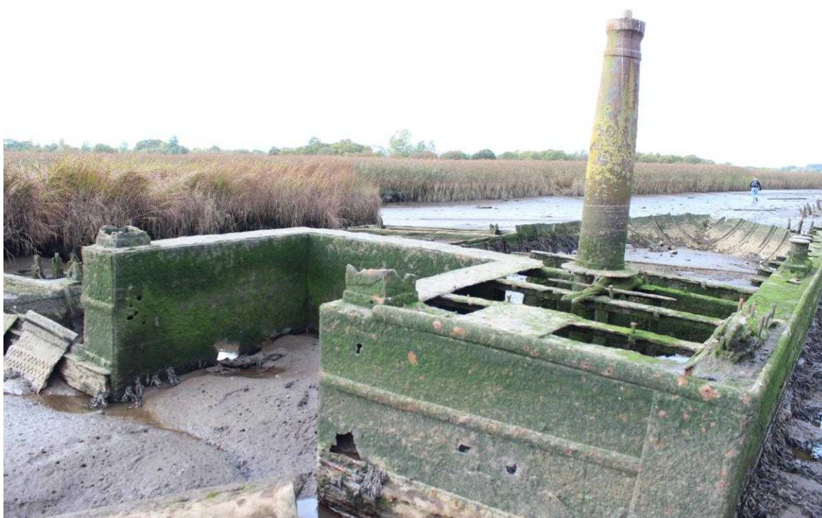
Figure 18: Detail of cutout at stern of Diving Bell Barge for housing diving bell.
