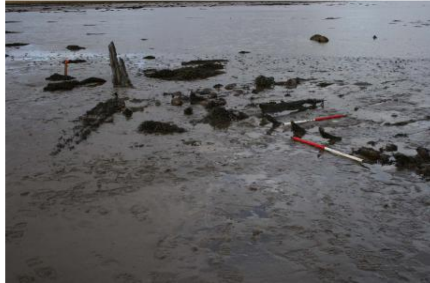
Figure 48: Wreck I, stern end of vessel showing stern post, detached stem and floors
