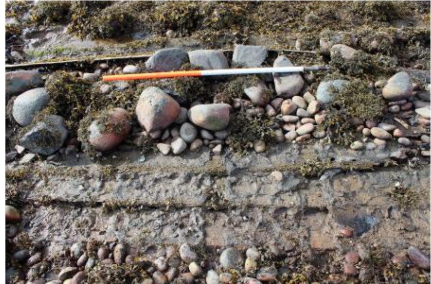
Figure 17: Wreck A, detail of planking showing clinker build and gaps in pitch showing frame spacing.
