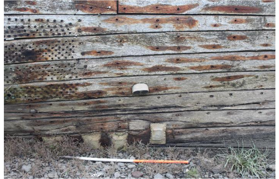
25. Wooden cutout with inset patch in strakes and lead patches near keel
