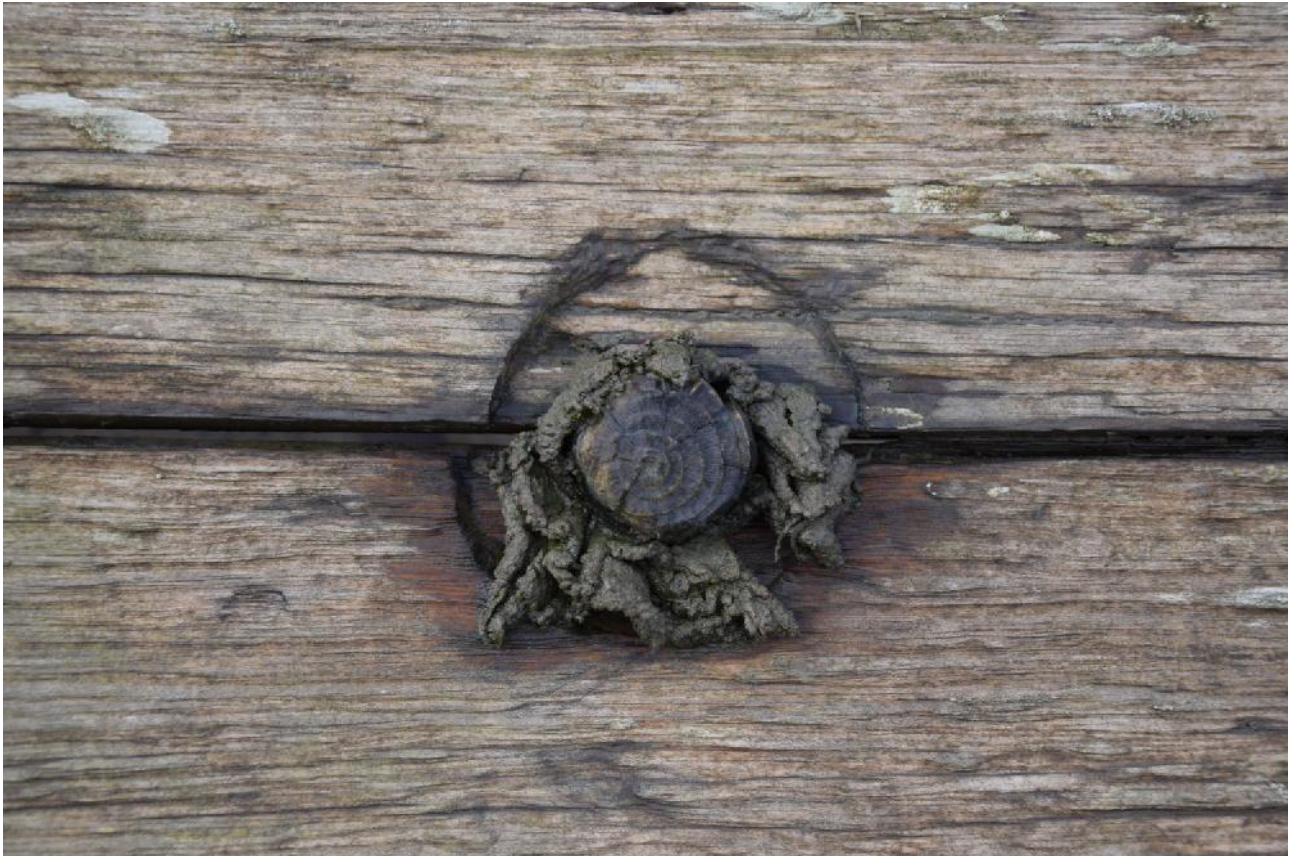
18. Fuelling hole in deck above engine
