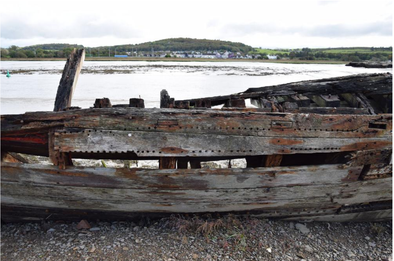
28. Rectangular cutouts at waterline on port side strakes on line of frames above wet-well, filled with wooden patches
