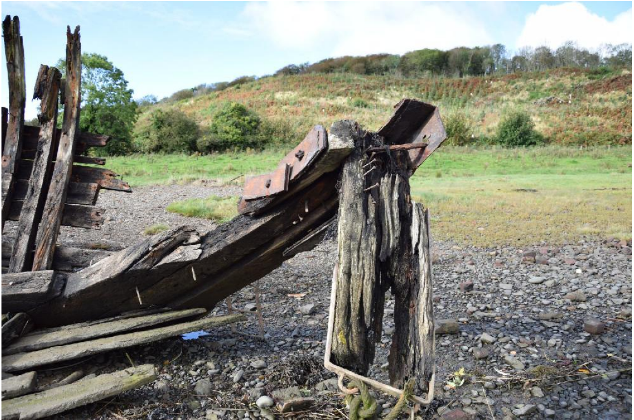
20. Stem post with collapsed upper timber and remains of steel plating
