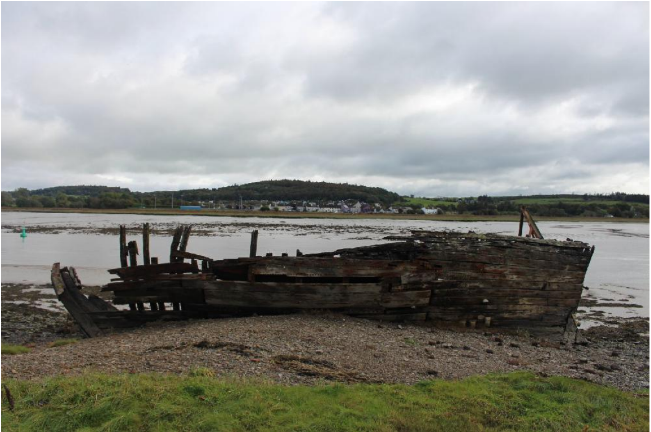
5. General view of the port side of the hull, showing the patched strakes in the wet-well
