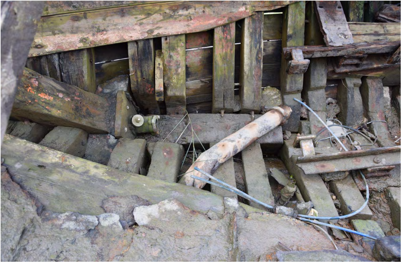
14. Aftermost floors cut down to accommodate engine and allow propshaft to pass through sternpost; poured concrete around base. Internal softwood timber fitted to internal face of sternpost to accommodate later stern gland associated with second engine
