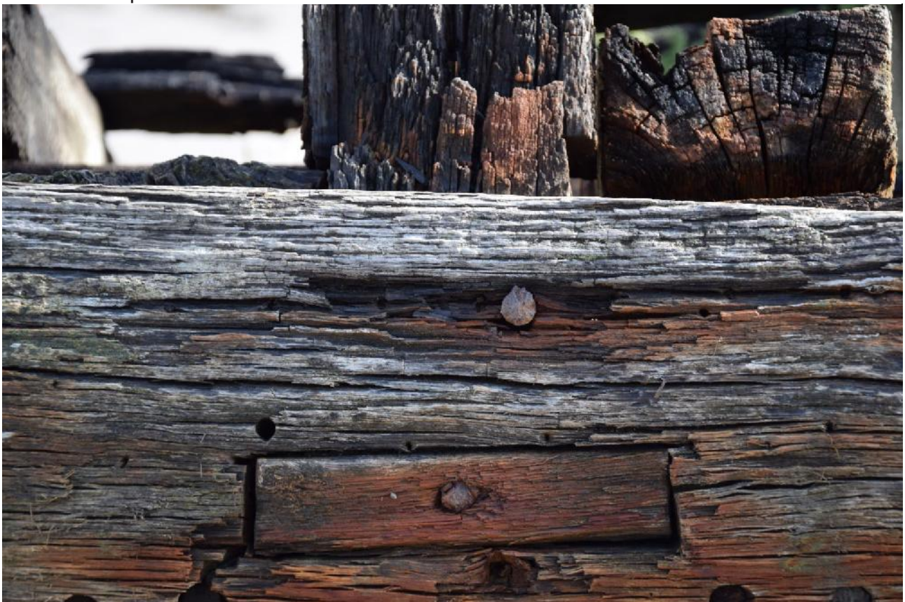
29. Detail of patched rectangular cutout in strake in line with frame above wet-well
