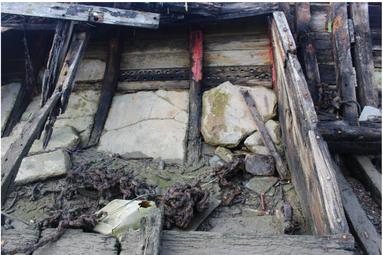
19. Concrete ballast over floors of the largest wet-well compartment, overlying the replacement strakes on the port side of the hull and likely contemporary with the installation of the later engine
