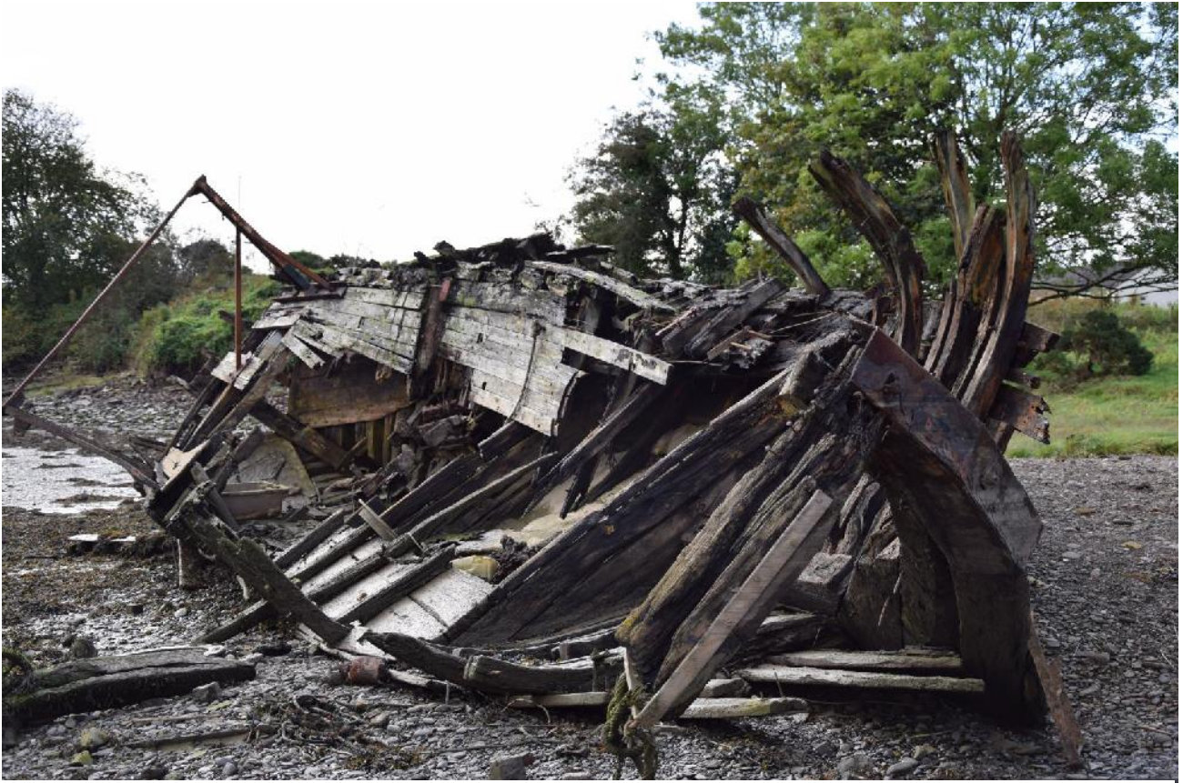
7. Bow area showing collapsed upper timber of stem post
