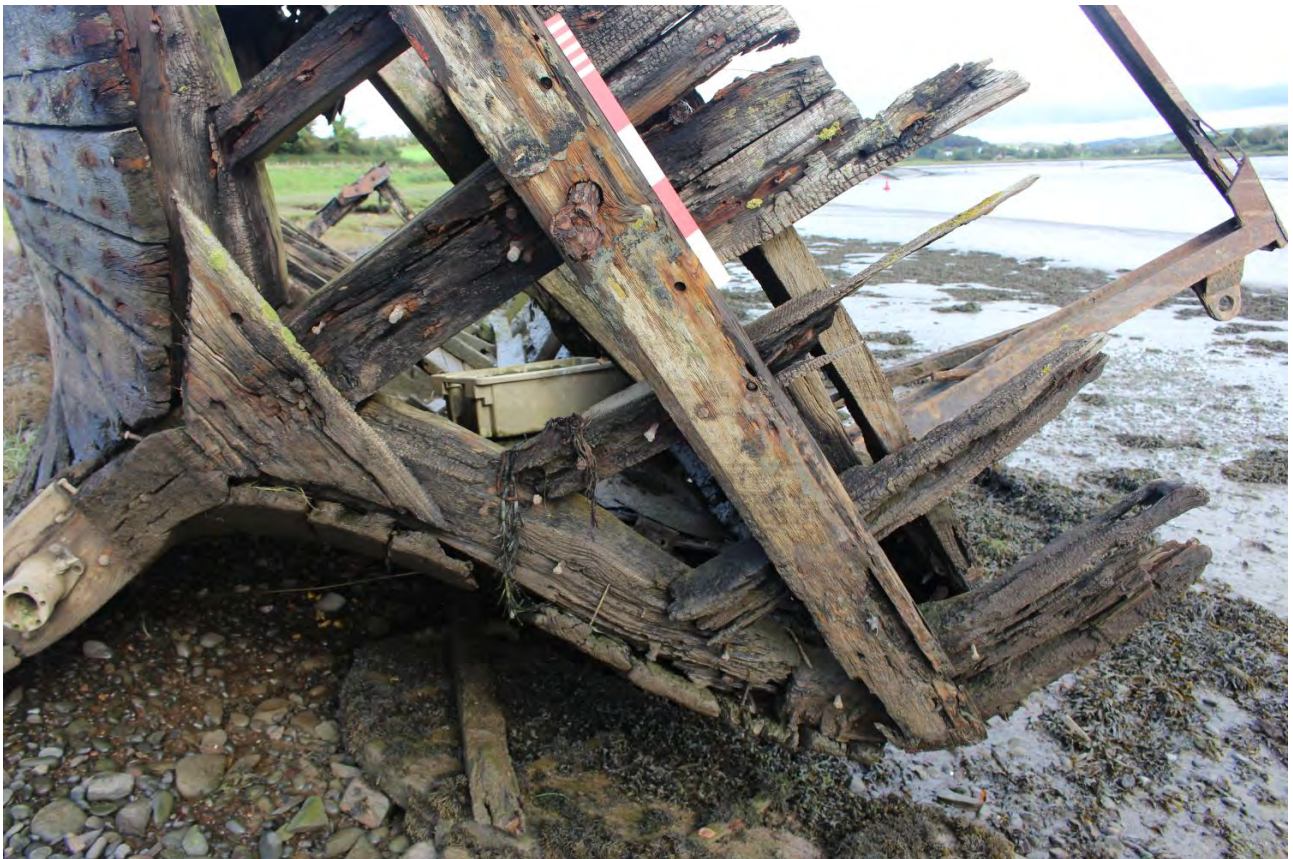
17. Transom with fallen rudder below with rehung offset setting for rudder to accommodate screw
