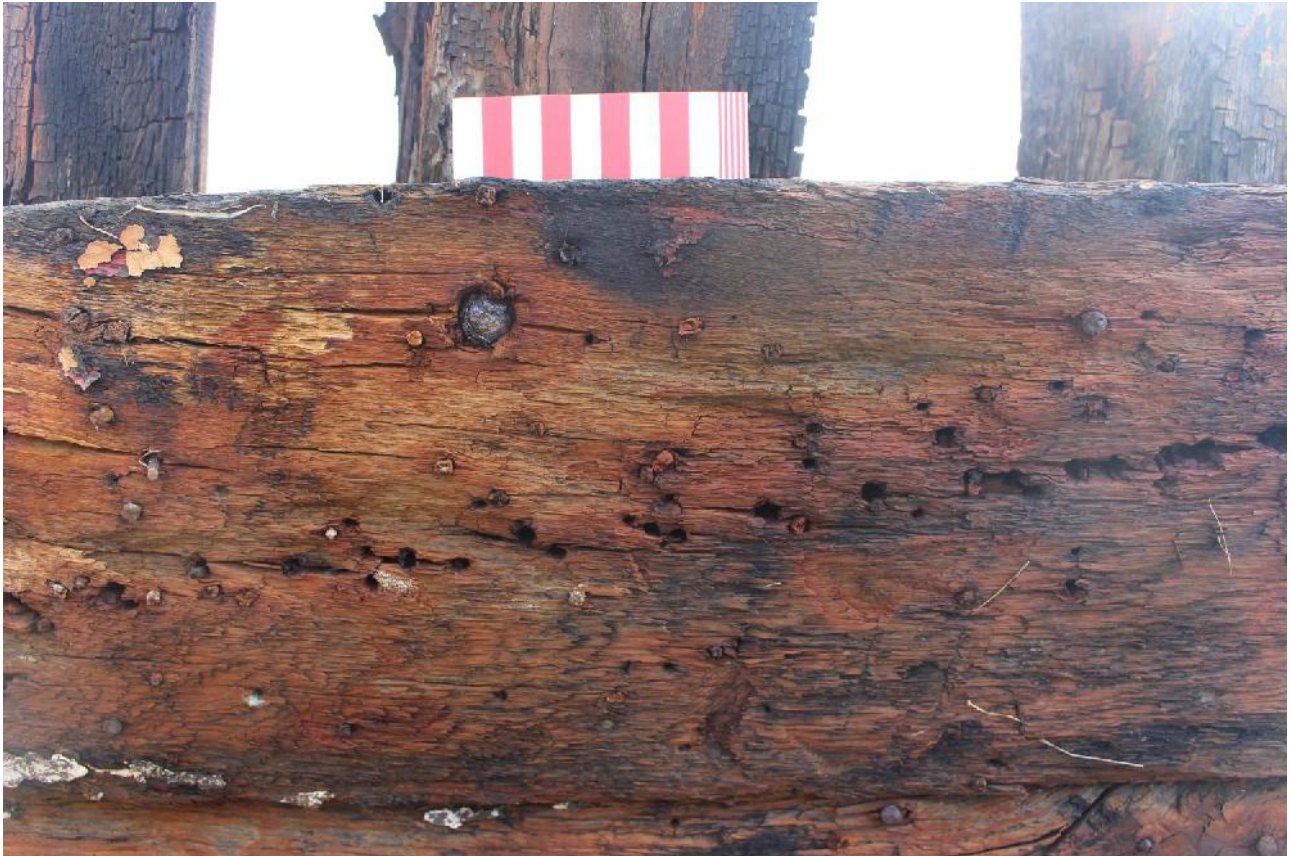
22. Iron staining and line of fasteners at waterline on port side bow
