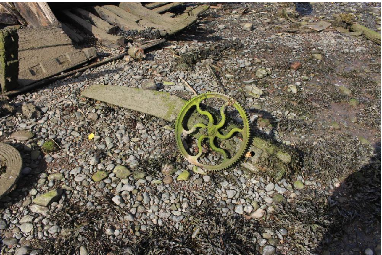
23. Collapsed samson post and windlass at bow
