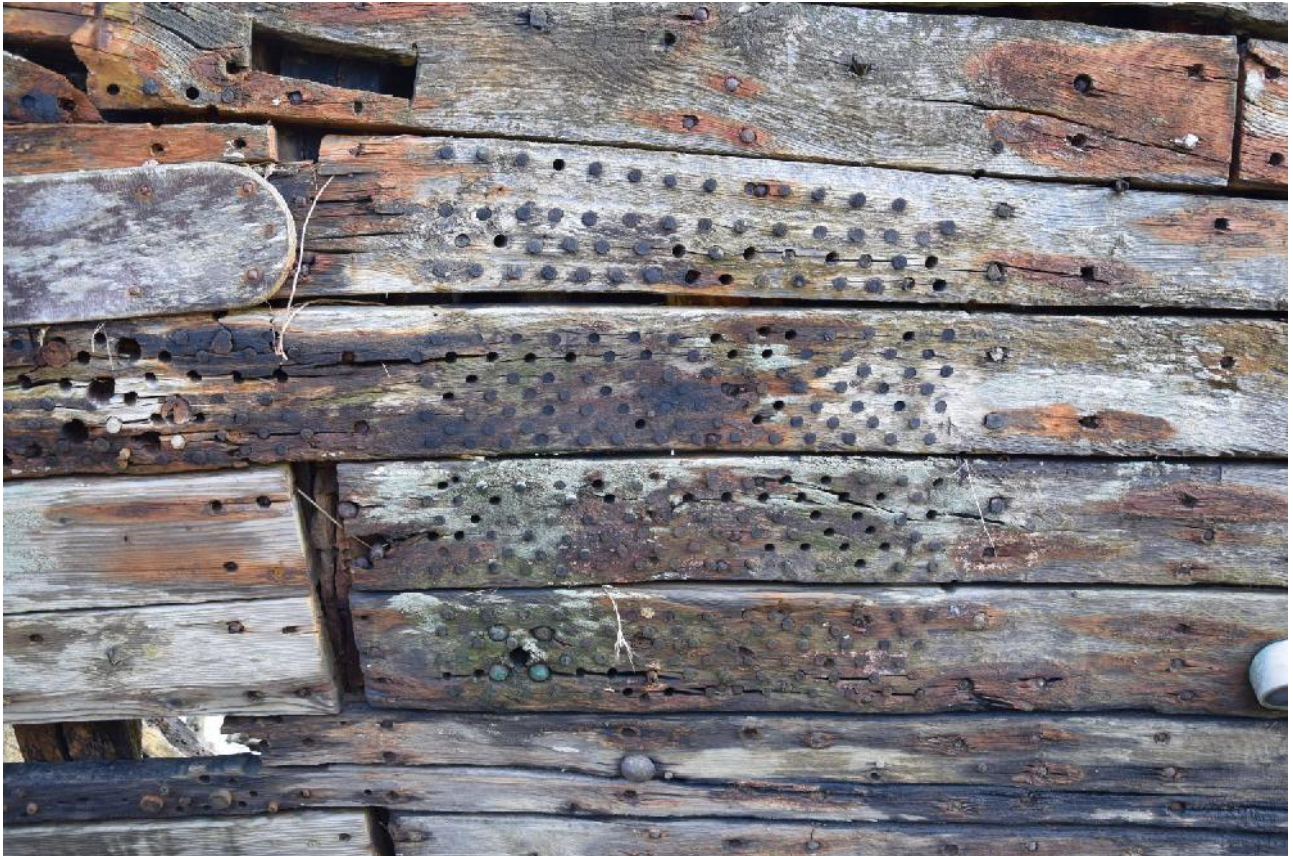
9. Detail of the holed strakes in the wet-well, and timber pegs plugging holes; replacement strakes in lower hull without holes. This repair post-dates the Fauna's time as a wet-well vessel
