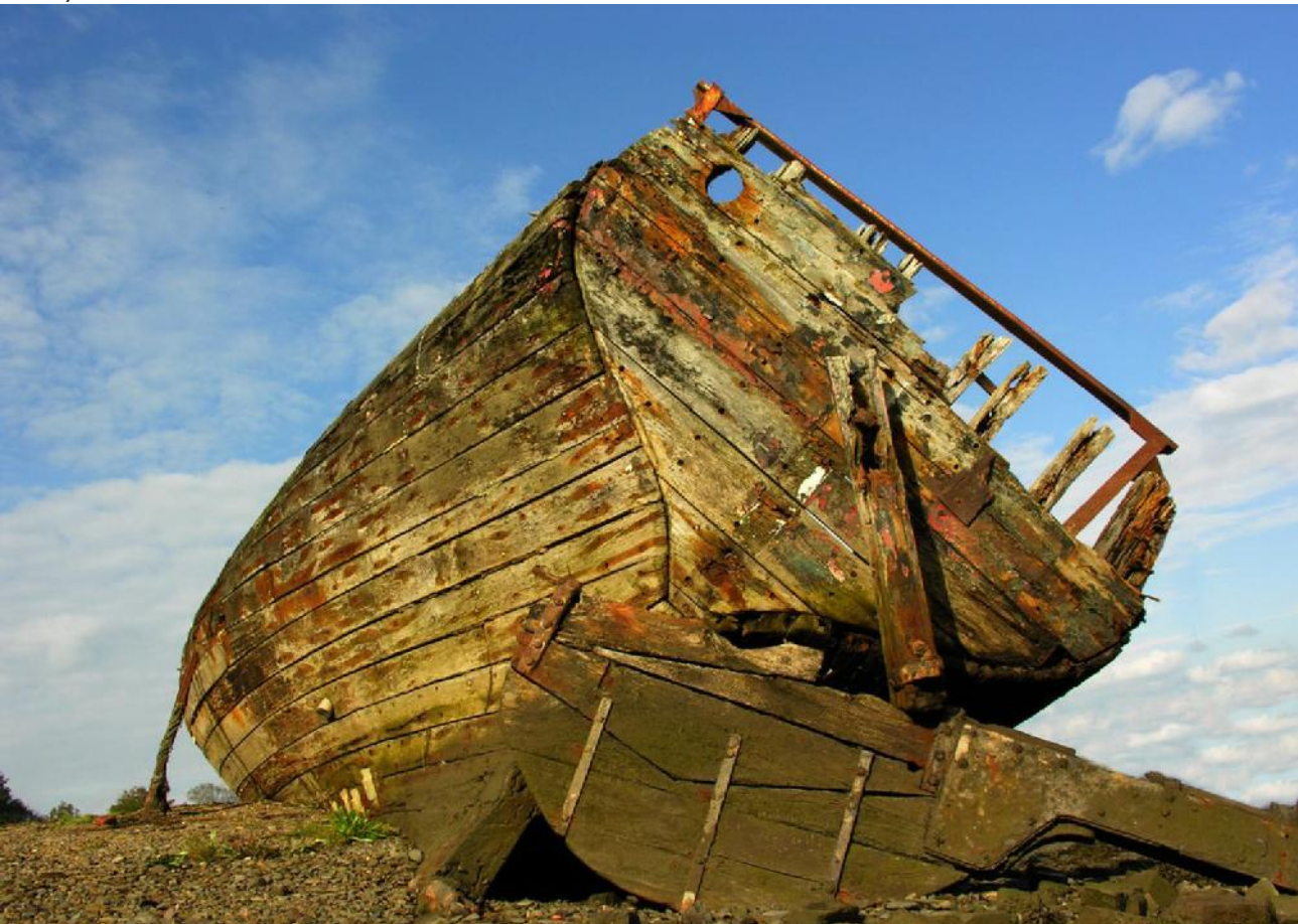
33. The stern showing the fallen rudder and plank mounted on transom to hold rudder offset to accommodate screw (Duncan McNeil, 2006)
