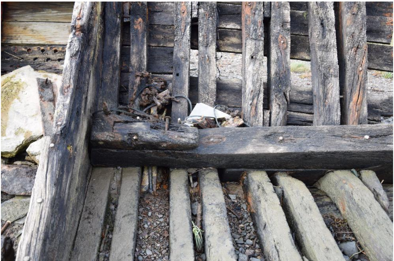
10. Mast step for a small foremast in the bow compartment, and forward bulkhead of wet-well on left with holed strakes visible
