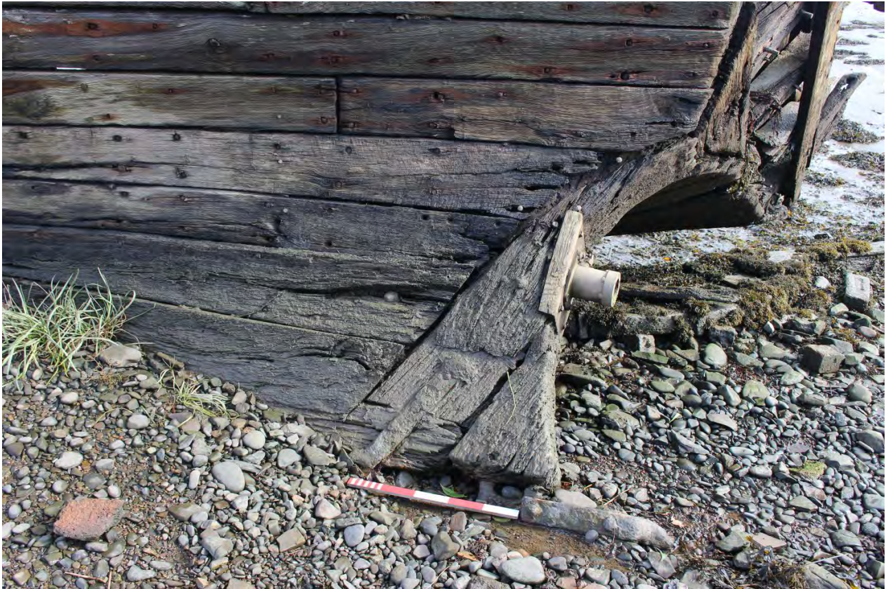
16. Cut in aft face of sternpost to accommodate screw propeller, with cheek fitted where prop-shaft cuts through, triangular extension for lower gudgeon for mounting of repositioned rudder. Stern gland mounted on softwood inset further cut into sternpost and cheeks
