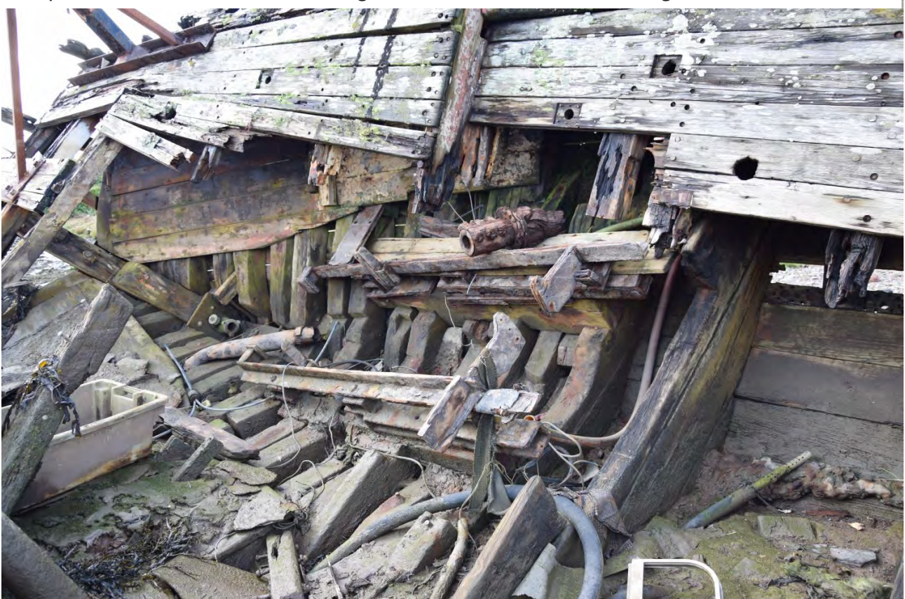
15. Aftermost two bulkheads of wet-well compartments cut down to accommodate engine. Earlier wooden engine bearers sitting on cut down floors with two pairs of steel engine mounts fitted on top and discarded Hardy Spicer joint.
