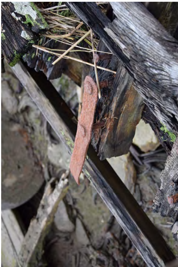
12. Chainplate attached to port bow frame
