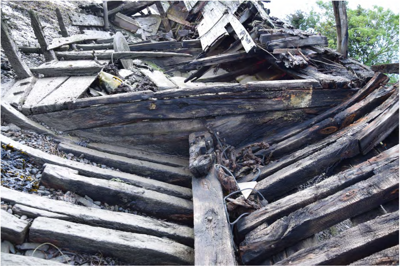
11. View along keelson across wet-well towards engine mounts
