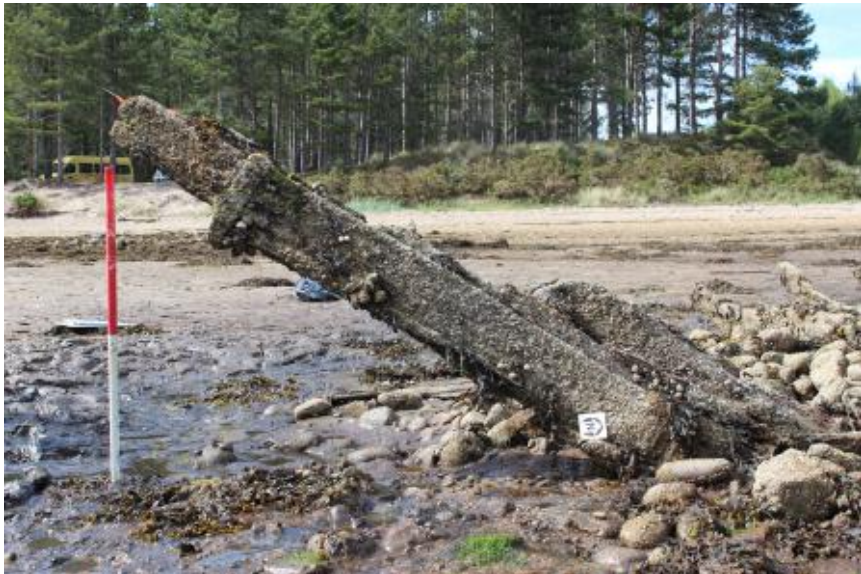
Figure 28: Wreck BB, detail of stern post with gudgeons
