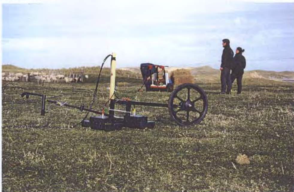
Figure 24 GPR equipment in use on Coll
